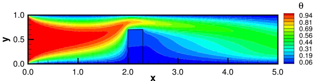
Figure 3. Temperature field for the base case ( $D_s = 1$ ).
