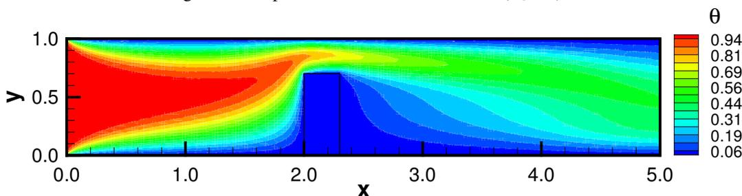
Figure 4. Temperature field for the case with  $D_s = 10000$ .
