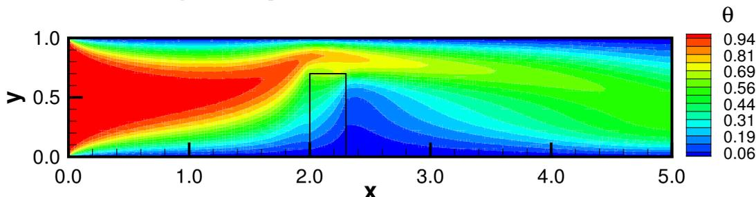
Figure 5. Temperature field for the case with  $D_s = 0.0001$ .
